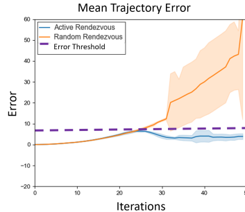
Fig. 4: Results for 50 robot simulation with trajectory error bounded at desired threshold. Y-axis Error= Err(x(t), \mathcal{E}_z(t)) and shaded region demonstrates standard deviation over 5 runs.
