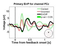
Fig. 7: This example ErrP was recorded during a closed-loop humanrobot interaction. FCz location is shown as the black dot on the scalp. Green highlights show where correct and incorrect trials differ significantly (p-val < 0.05, Wilcoxon signed rank test, corrected).
