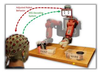
Fig. 1: The robot is informed that its initial motion was incorrect based upon real-time decoding of the observer's EEG signals, and it corrects its selection accordingly to properly sort an object.
