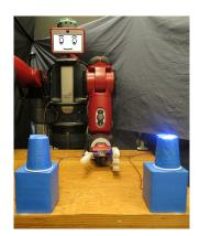
(a) The subject is seated directly between two possible targets with indicator LEDs - here, the right LED indicates the correct target. Curtains surround the test area and subject to minimize distractions.
